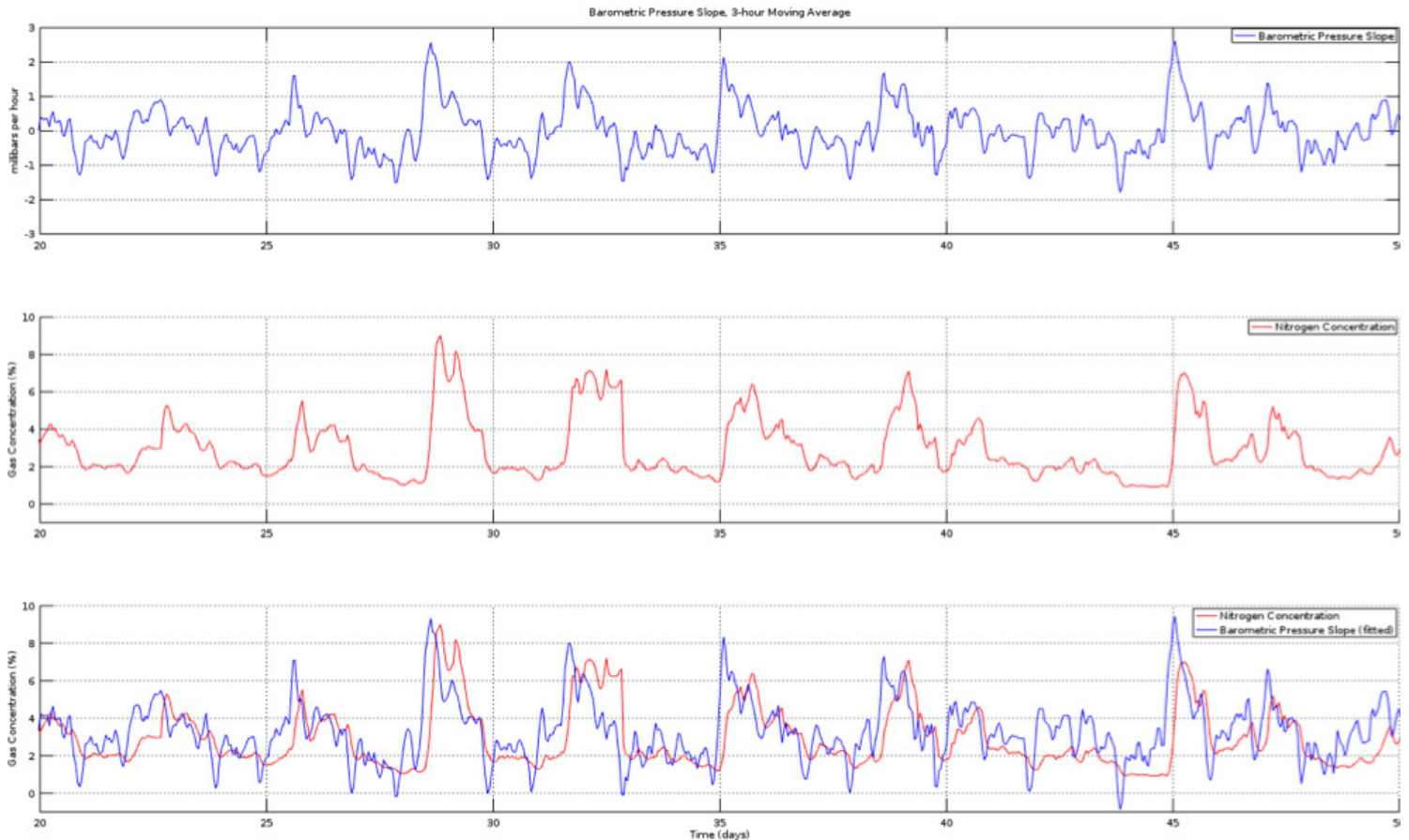
Figure 3: Nitrogen concentration in sales gas is proportional to the rate of barometric pressure change. For a 30-day period pre-automation, a 3-hour moving average of barometric pressure, with a 4-hour shift applied, is shown in blue. Nitrogen concentration in the sales gas is shown for the same period. Strong visual correlation observed; statistics for the full winter period pre-automation are shown in Figure 8 .
