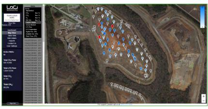
The WellWatcher® platform and user interface provides real-time data and visibility across the landfill gas collection system.
