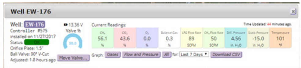
Photo 1: Loci Controller which provides real-time gas composition monitoring and algorithm based well tuning, installed on a gas collector at Oklahoma City Landfill.
