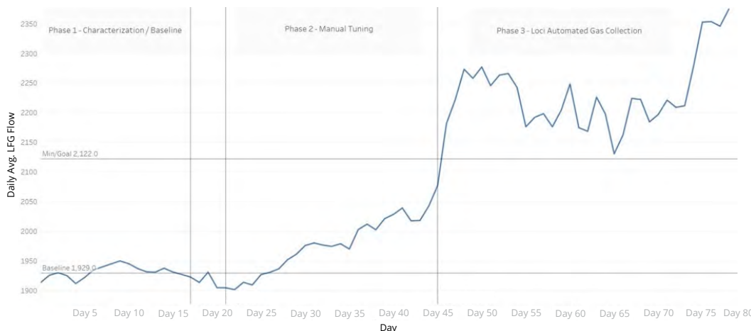
Figure 1: Increasing LFG flow from automated tuning
