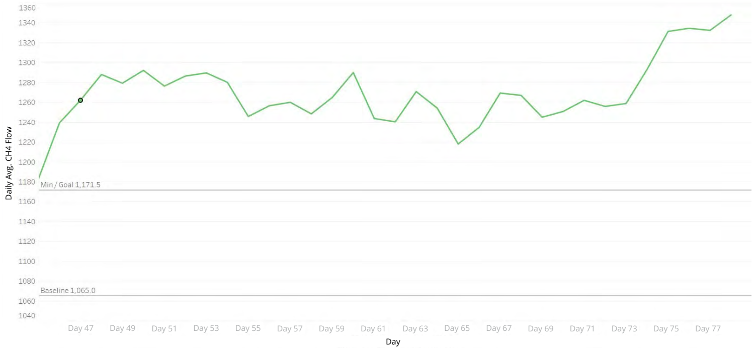
Figure 6: Phase 3 CH 4 flow – consistently above targeted goal of 1171 SCFM
