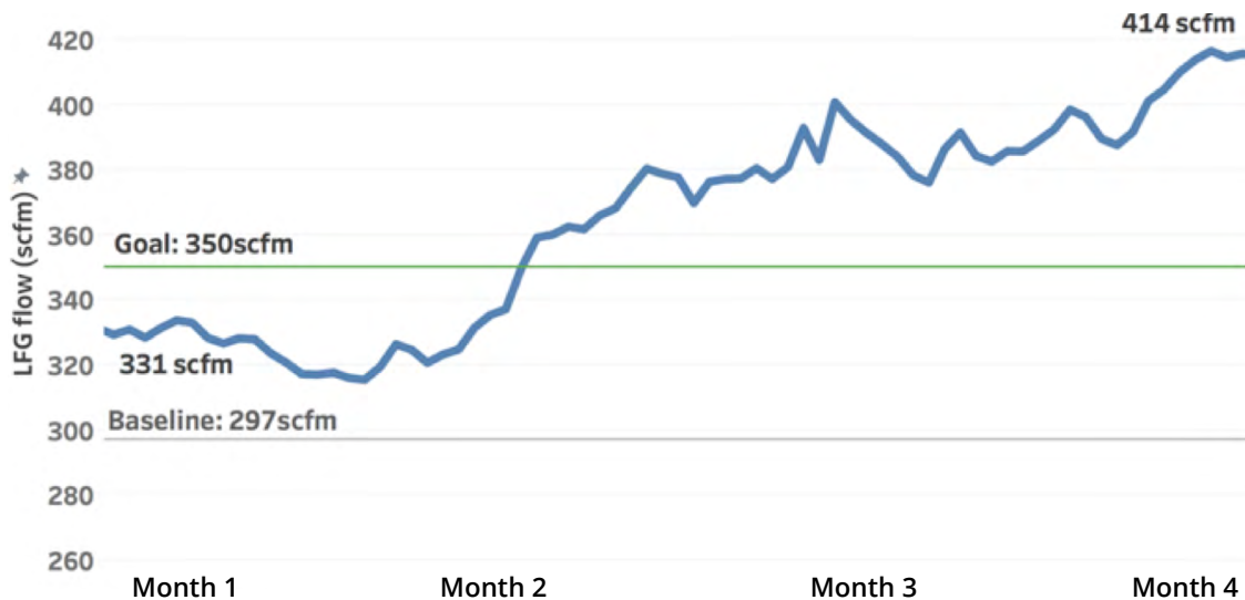
Figure 1: Increased LFG flow after installation of Loci Controls system
